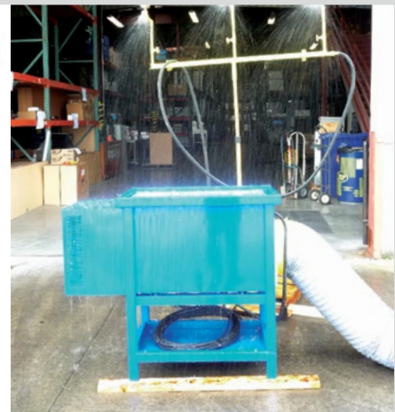
Outdoor rating inlet rain baffle with electrical and cord cover
